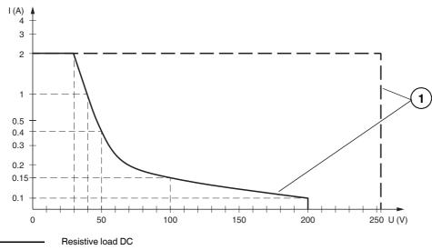
Resistive load AC max. 10<sup>5</sup> switching cycles
